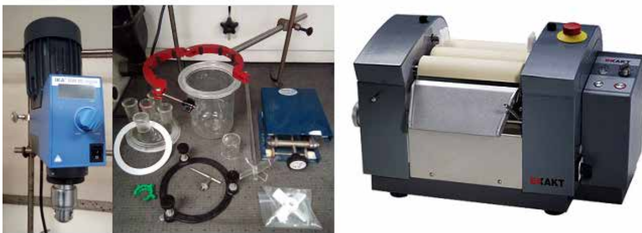
Figure 1: Processing equipment for grease sample production: (left) kettle-style chemical reactor and peripherals with mechanical overhead stirrer, and (right) 3-roll mill.
