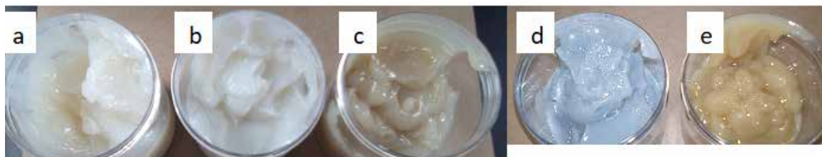
Figure 6: Grease samples formulated using (left) G1BO with (a) 12-HSA, (b) 12-HSA with azelaic acid, and (c) MFA1, and (right) G2BO with (d) 12-HSA, and (e) MFA1.
