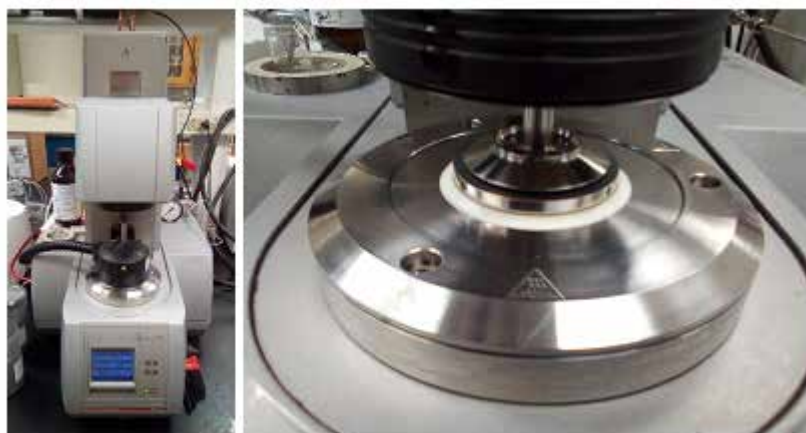
Figure 3: Modular compact rheometer (left) and full instrument profile (right) sample stage with a 50 mm parallel plate geometry.
