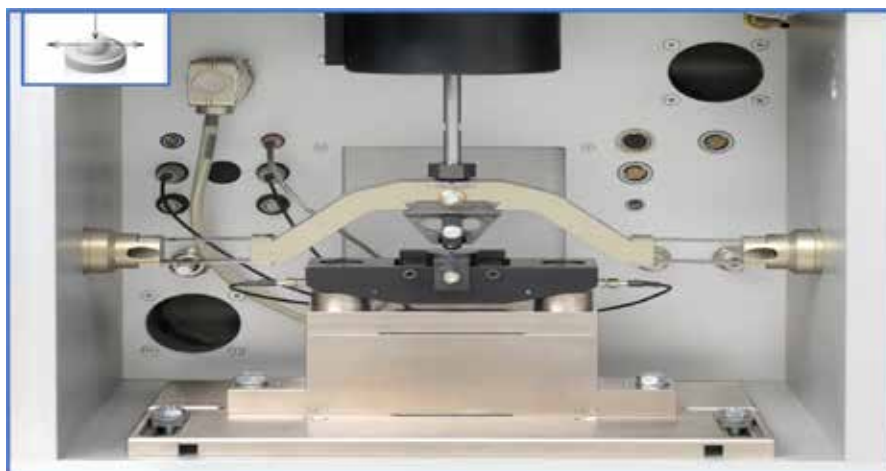
Figure 1 SRV® oscillation chamber
