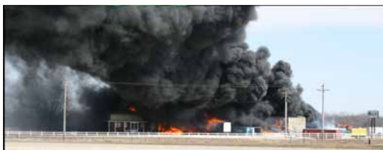
Figure 1 In 2007, a heat transfer fluid leak started a chain of events that led to a fire at a biobased grease plants
