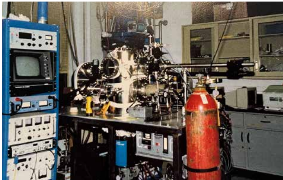
Ray used this ultra-high vacuum chamber to study boundary layer formation on metal surfaces in a laboratory at the University of Illinois at Urbana-Champaign. (Photograph circa 1990, originally published on page 17 of Ray's Ph.D. Thesis).
