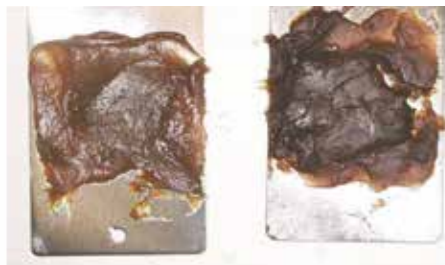
Figure 8 – Appearance of 3.8-year aged & 70 Mrad irradiated CC Grease B before and after exposure to LOCA conditions
